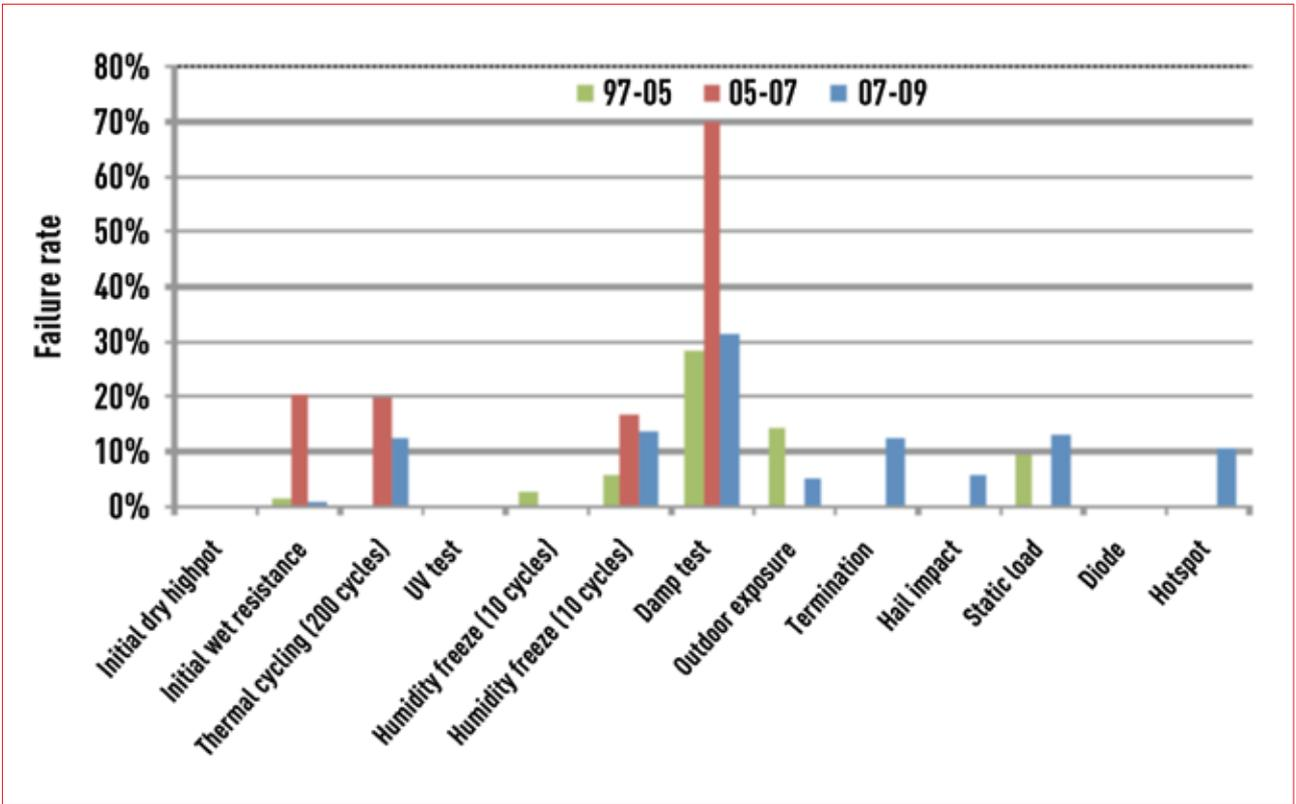
Figure 2. Failure rate comparison of thin-film modules for 1997-2005, 2005-2007, and 2007-2009.
