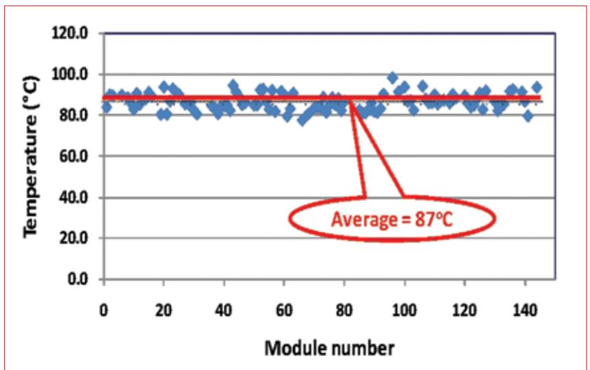
Figure 3. Normalized cell temperature, standard testing (ambient temperature 40°C; irradiance 1000W/m<sup>2</sup>).
