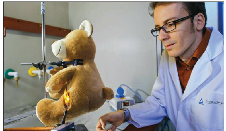
In this laboratory setting, a flammability test is administered.
