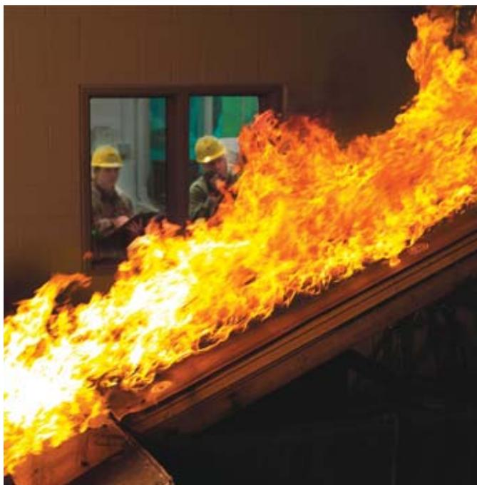
**Figure 1. A PV Panel Being Tested to ASTM E108 Fire Test at the Intended Installed Slope**
