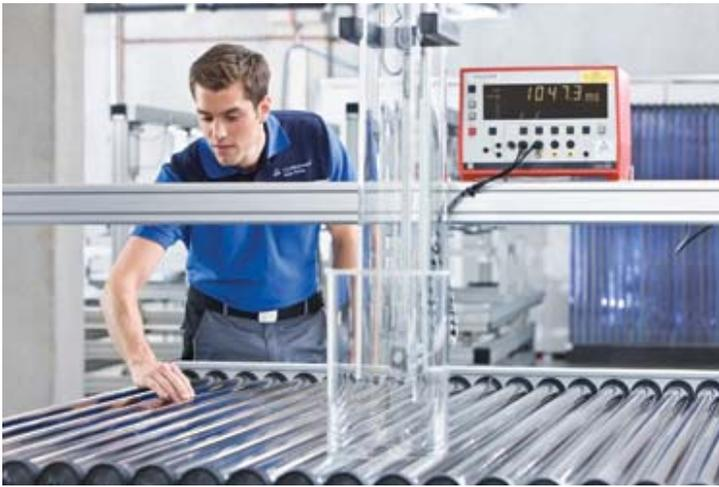
**Figure 2. Hail Impact Testing on a Solar Collector**
