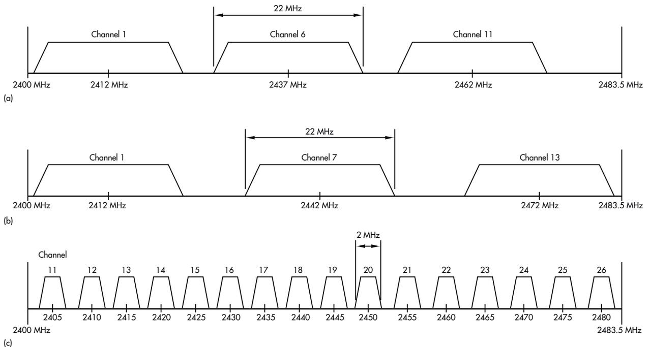
The operational channels for 802.11 Wi-Fi and 802.15.4 ZigBee overlap, which could cause interference problems. However, the RF4CE standard includes frequency agility in the remote control and its targets to mitigate this problem. Shown are the channel selections for IEEE 802.11b North America, non-overlapping (a), IEEE 802.11b European, non-overlapping (b), and IEEE 802.15.4, 2400-MHz PHY (c). (source: IEEE 802.15.4-2003 Specification)
