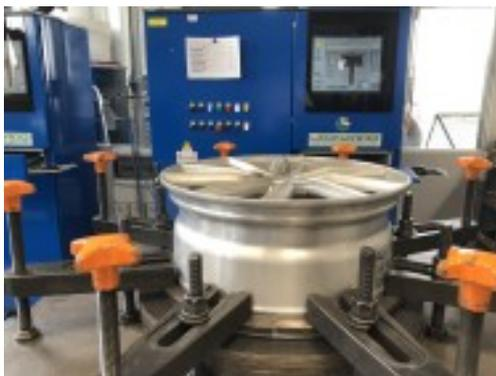
A further increase in the capacity of tests that can be carried out is represented by the installation of a new double station Radial Rolling Fatigue test machine, which is therefore able to test 2
