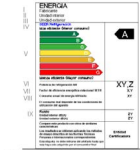
Figure 1-1: Design of the energy efficiency label for air conditioning appliances with minimum energy efficiency
