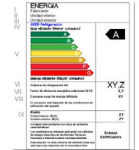
Figure 1-1: Design of the energy efficiency label for refrigerating appliances with minimum energy efficiency
