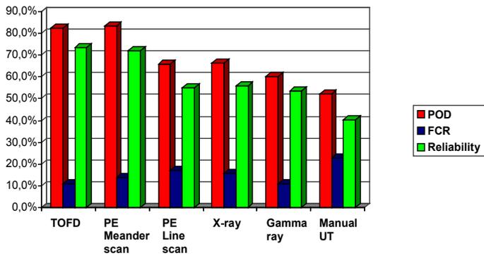
All plates were examined with the techniques shown here and later the results were verified by destructive testing. Collected data resulted in manual pulse-echo ultrasonic examination detecting slightly over 50% of the defects present. However, in about 23% of the cases, manual pulse-echo reported defects where no irregularities could be confirmed (FCR).
