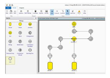
PEL Adrian calculates flows and pressures for high velocity, compressible gases in a network and is relevant for the modelling of relief streams
