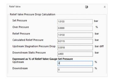
For bursting disc systems the relief pressure and the exit pressure, along with the frictional losses in the pipe and across the disc can be modelled to determine the system capacity.
